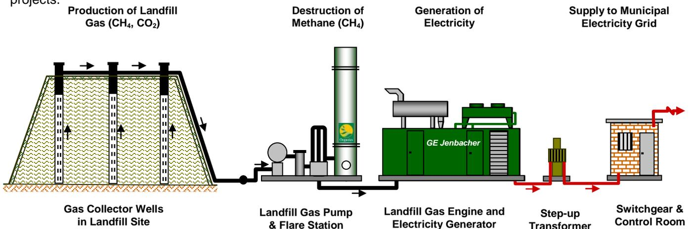
**Schematic Layout of Landfill Gas-to-Electricity Project**
