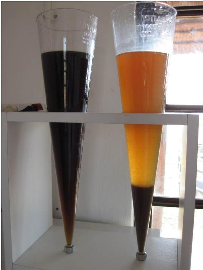
**Clearer Waters:** The Imhoff cone test on the left illustrates the difference between raw landfill leachate which is fed into the leachate treatment plants, and on the right a sample of the 'mixed liquor' from the sequencing batch reactor (SBR) where the top 'supernatant' is then sent to the reedbed for final 'polishing' treatment. The sludge in the bottom of the cone are the plant work-force – the activated sludge of bacteria that effects treatment!
