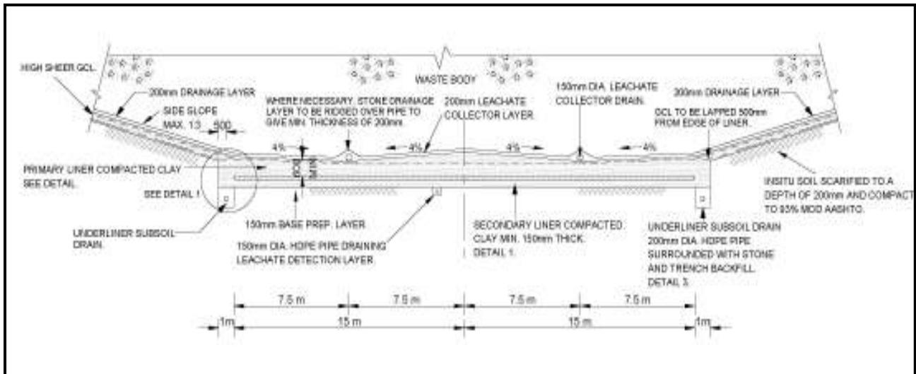
**Figure 5 – Side Slope Liner**
